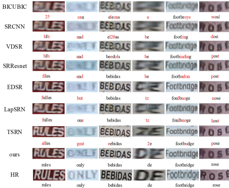
Fig. 10. Different SR methods’ visualization and recognition results: the last row represents an HR image, “ours” represents the proposed model (TSRMAN), and “red” presents misrecognition.
